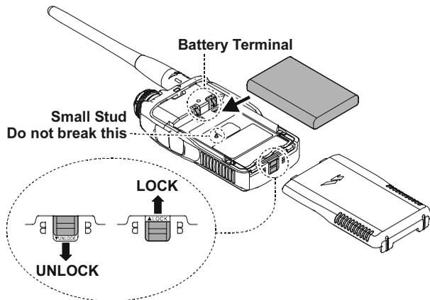
**Important Note:** *There is a small stud in the Battery Compartment of the VX-3R/E. This stud is a switch for the battery detection. Please be careful not to break this stud while changing the battery.*
