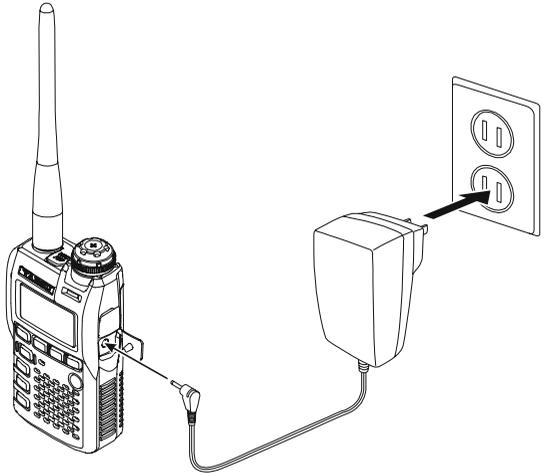
While the battery is being charged, the display will indicate “CHGNG” and the **TX/BUSY** indicator will glow red. The S-meter will deflect according to the charging status.
