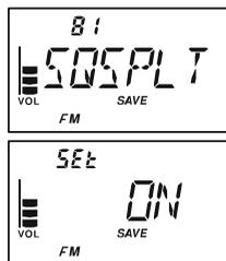
When the Split Tone feature is activated, you can see the following additional parameters after the “MESSAGE” parameter while selecting the Set Mode Item 79: SQ TYP:
