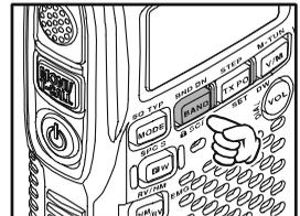
If you wish to reverse the direction of the scan (i.e. toward a lower frequency, instead of a higher frequency), just rotate the **DIAL** knob one click in the counter-clockwise direction while the **VX-3R/E** is scanning. The scanning direction will be reversed. To revert to scanning toward a higher frequency once more, rotate the **DIAL** knob one click clockwise.
