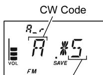
8. Press the **[F/W]** key to begin generating the selected code characters the designated number of times (Only the speaker CW sidetone is heard, the radio does not transmit).
