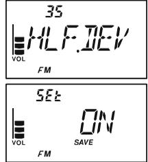
*The "normal" setting for the deviation (when this Menu Item is set to "OFF") is  $\pm 5$  kHz.*
