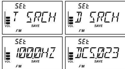
6. When the radio detects the correct tone or code, it will halt on that tone/code, and audio will be allowed to pass. Press the [BAND] key to lock in that tone/code, then press and hold the [TXPO] key for one second to exit to normal operation.
