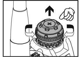
If you press the **[F/W]** key momentarily, then rotate the **DIAL** knob, frequency steps of 1 MHz will be selected. This feature is extremely useful for making rapid frequency excursions over the wide tuning range of the **VX-3R/E**.
