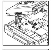
7 Refer to the figure on the right to mount the FVS-2 Caution Check the direction of the connector and plug the FVS-2 in all the way to the back.
