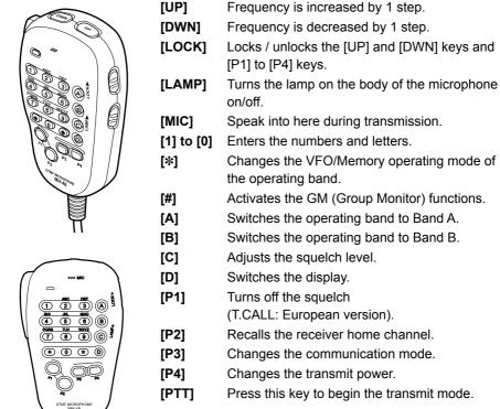
Tip — Preferred functions can be assigned to buttons [P1] to [P4]. Select using the [CONFIG]→[10 MIC PROGRAM KEY] in the set-up menu.
