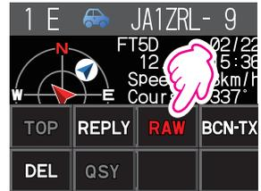
Details of RAW packet data display screen
