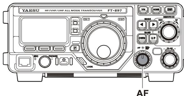
When operating in the “DIG” or “PKT” modes, you may set the AF knob to any comfortable setting, or even all the way off, because the output from the **DATA** jack is a fixed-level audio signal.
