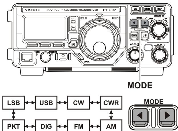
where “CWR” is “CW-Reverse,” using the opposite sideband from the “default” BFO injection sideband (in most cases, the default injection sideband is on the “USB” side); “DIG” is an AFSK-based Digital mode, set up per Menu Mode No-038 [DIG MODE]; and “PKT” represents either 1200 or 9600 bps FM packet.
