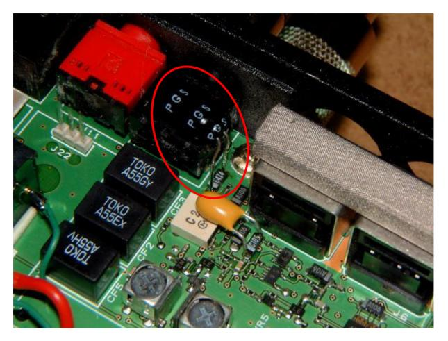
Here you can see how I easily added a normal 4,7µF electrolyt in parallel.
