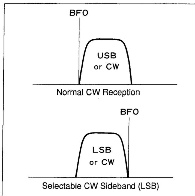
Using this feature, you may freely tune LSB voice and CW signals *from within the same mode*, and even select the narrow CW filter (if installed) *without having to change modes and re-tune your desired signal*. Normal USB and LSB reception is still possible as before, however, when in CW mode, the selected CW sideband offset will automatically take effect.
