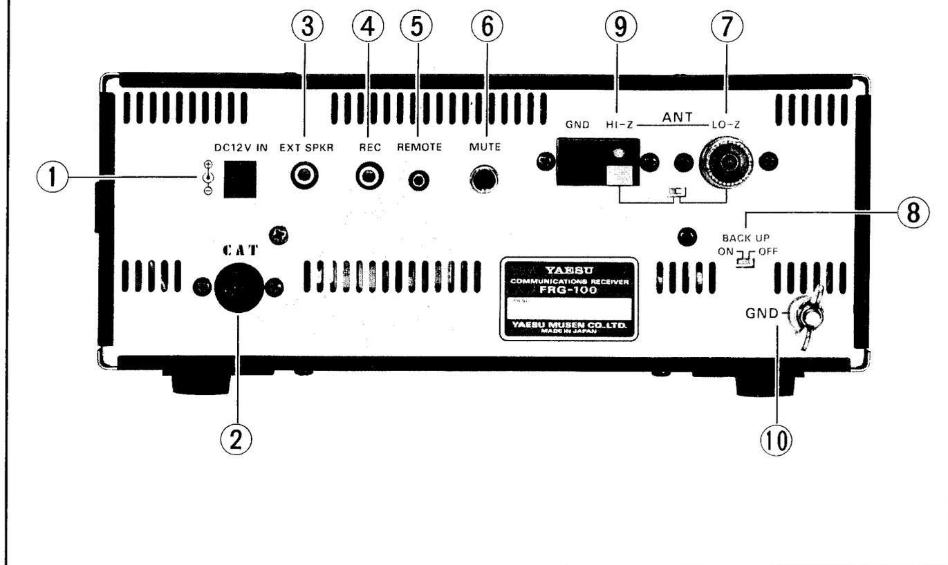
**1 DC 12 V IN** This is the 13.8-volt DC power connector. Be sure to use a coaxial-type barrel plug. A regulated power supply capable of providing at least 2 amps is recommended. Be sure to observe proper polarity and ensure that the center conductor is wired + (positive) and the outer conductor is — (GND).
