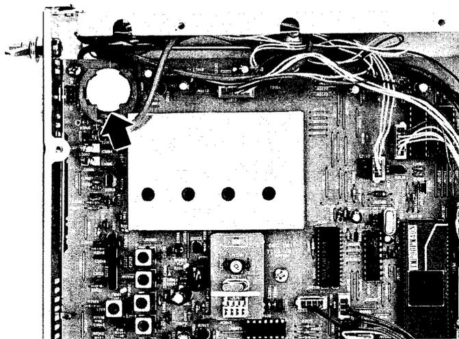
Fig. 9 Lithium Battery Location
