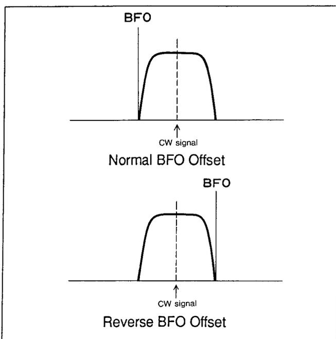
The Reverse BFO Offset can only be enabled from within the Selectable CW Sideband mode previously explained. If you are tuned to a CW signal receiving interference, perform the following steps.
