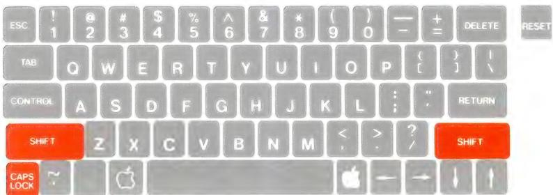
Figure 2-3. CAPS Lock and SHIFT Key
