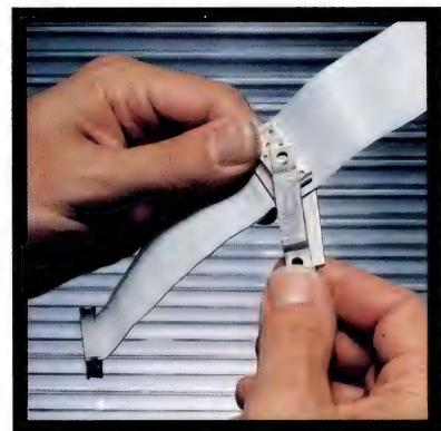
6. Feed the cable back through the back panel opening until you can fit the raised side of the clamp in the opening.
