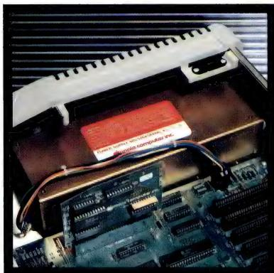
Now that you have had a good look at the computer, it's time to install your cards and peripheral devices. The standard procedure for doing this follows. The **80-column text card** is shown as an example:
