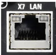
The LAN port (RJ-45) at the rear panel is a 10/100/1000Base-T port. Use this port to integrate the R&S EB500 in a local area network (LAN), primarily for remote-control purposes.
