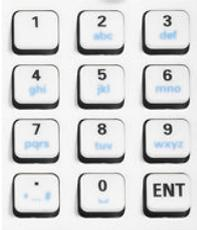
The keys in the data entry keypad are used to enter numbers and letters. Data entry keys are only enabled if an editable field has been selected for entry mode. This can be achieved in the following manner:
