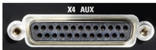
**X3 AUX AUDIO** is a 25-pin D-Sub female connector with the output of different audio signals. There are also some special trigger inputs on this connector. Use this connector if you want to record the analog audio signal of the R&S EB500
