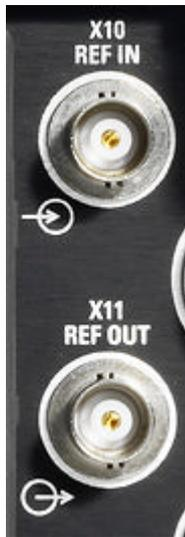
**X10 REF IN** is a BNC input for an external reference frequency. Use this connector to synchronize the receiver with a frequency normal.
