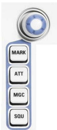
After pressing either one of the keys MARK, ATT, MGC or SQU, the SELECT rollkey will act on behalf of the respective Marker, Attenuation, (Manual) Gain Control or Squelch function of the receiver.
