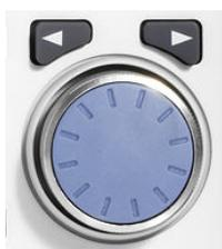
The navigation keys consist of one rollkey: the "Main Rollkey" or ROTARY KNOB and two arrow keys: CURSOR LEFT and CURSOR RIGHT.
