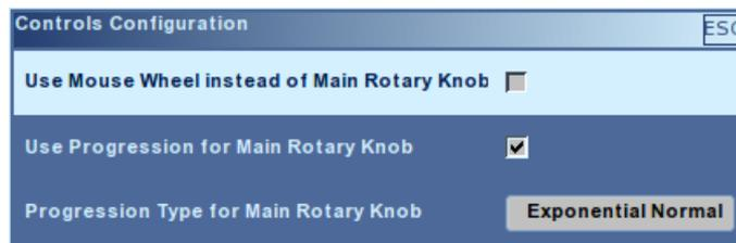
This dialog is used to configure the R&S EB500's controls, i.e. its keys and knobs. For instance you can set the device to produce a sound when a key is pressed. You can also set the direction for the main rotary knob (ROTARY KNOB) as well as its progression.
