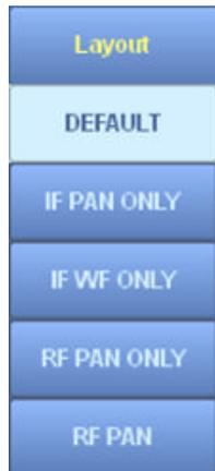
When pressed, the "Layout" softkey will open a vertical selector with the different layout options.
