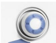
Pressing the SELECT knob (see: "[Receiver Control Keys](#)" on page 26) activates or deactivates a single range marker. Non-selected range markers are displayed in a translucent color (red or purple). Measurement output fields are displayed along the upper edge in the respective range-marker color.
