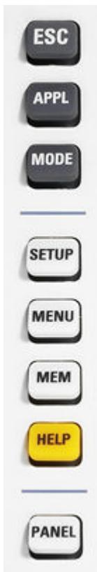
At the left side of the display we find the utility keys: these are keys that provide the operator with menus and dialogs to configure settings, and shortcuts to change the R&S EB500 into different receiver application or operation modes. There are also "Help", "Escape" and "Panel focus" keys.
