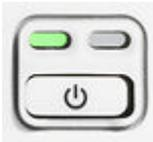
The STANDBY key toggles between STANDBY and READY state and shuts down the R&S EB500. See [chapter 2.2.7, "STANDBY and READY"](#), on page 21 for an explanation of the LED colors related to the state of the device.
