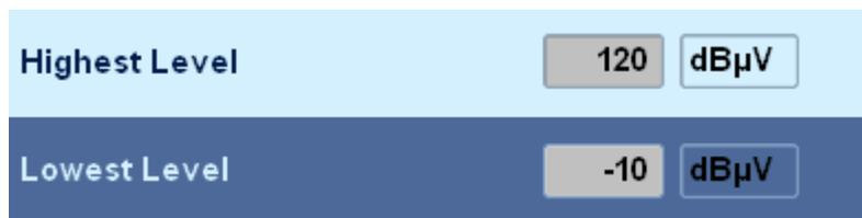
The scale of the RF panel can be set by activating the "Highest Level" and / or "Lowest Level" fields and the values can be changed, by using the ROTARY KNOB or the numeric keys. A selector bar will accompany the selection with the options dBµV or dBm as well as +/- and Backspace options.
