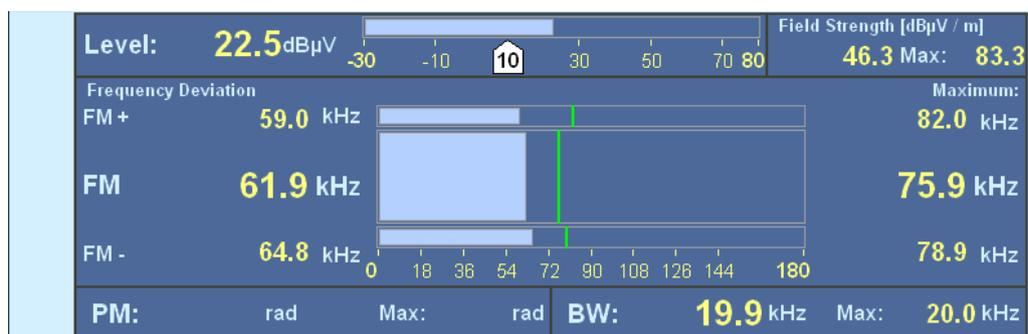
Fig. 3-10: ITU Panel: Frequency deviation measurement.
