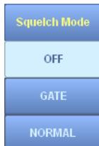
Press the "SQU MODE" button to select or turn off the squelch mode. If the DF squelch is turned off, it is not shown in the DF panorama or the polar panel.
