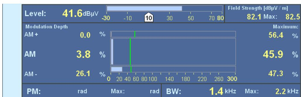
Fig. 3-11: ITU Panel: Modulation depth measurement.
