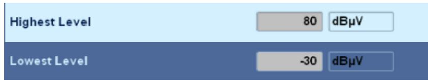
The scale of the IF panel can be set by activating the "Highest Level" and / or "Lowest Level" fields and changing the values, using the ROTARY KNOB or numeric keys. A selector bar will accompany the selection with the options dBµV or dBm as well as +/- and Backspace options.
