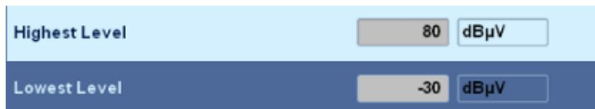
The scale of the DF panel can be set by activating the "Highest Level" and / or "Lowest Level" fields and the values can be changed, by using the ROTARY KNOB or the numeric keys. A selector bar will accompany the selection with the options dBµV or dBm as well as +/- and Backspace options.
