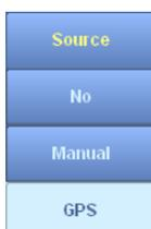
Use this field to specify the declination source. You can use the value supplied by a connected GPS receiver or you can enter a value manually. A related selector shows the available options. Available options are "No", "Manual" and "GPS".
