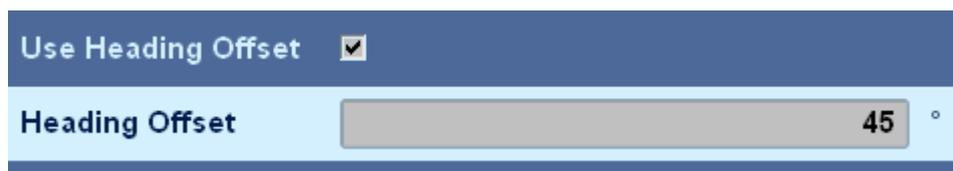
Set a check mark next to "Use Heading Offset" label if you want the offset for the selected compass to be used for the "North Correction" (see [SYSTEM:COMPASS:HEADING:OFFSET](#) on page 323). This will also enable the field "Heading Offset" for editing. Use this field to set the desired offset for the selected compass. You can enter a value between 0° and 359.9°.
