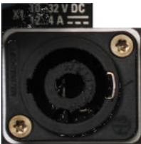
The DC power connection X1 is located at the top left corner of the R&S EB500 rear panel. With the DC power connected, the R&S EB500 is in STANDBY or READY state, depending on the state of the STANDBY toggle switch at the front panel of the R&S EB500 when it was last switched off. The standby power is below 0.8W.
