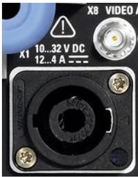
Standard Speakon NL4FX socket for DC power input. Socket accepts 10~32 VDC on pin 1+ and ground on pin 1- of connector. Power requirement as indicated. Refer to [chapter 2.2.5.1, "Connecting to the Power Adapter"](#), on page 20 for instructions on connecting to the power adapter using the Speakon NL4FX connector.
