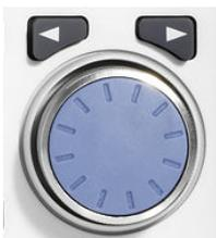
The DDC currently being configured is highlighted in yellow. Once you have activated the panel, you can select the desired DDC using the CURSOR LEFT / CURSOR RIGHT keys. Use the ROLLKEY to change the receive frequency of the selected DDC.
