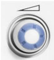
The volume of the speaker and headphones is adjusted with this knob. Pressing the knob will toggle the speaker mute. Headphones remain active when the speaker is in mute position.
