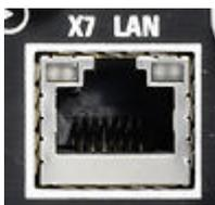
You can connect a LAN cable to the LAN port (X7) on the rear panel of the R&S EB500.
