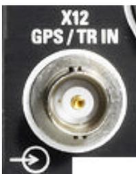
**X12 GPS/TR IN** is a BNC connector for an external 1 sec trigger pulse, e.g. from a GPS device.
