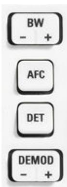
BW selects the demodulation bandwidth (between 100 Hz and 20 MHz).
