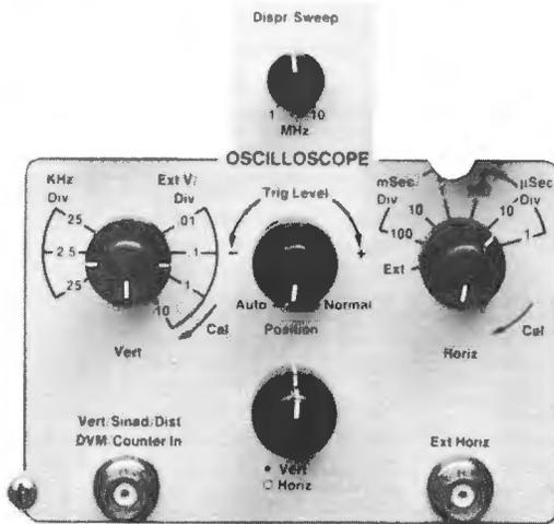
FIGURE 3-40. OSCILLOSCOPE SECTION
