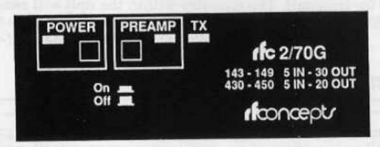
Power LED: This LED will illuminate when power is applied to the amplifier.
