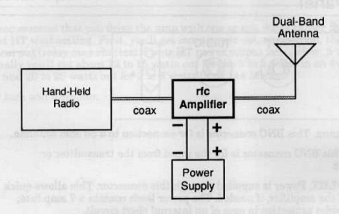
CAUTION: If you are expecting to operate both bands, you'll need to use a dual-band antenna. Check with your dealer. If you operate dual band without a dual-band antenna, you could damage the power transistors if you key up on the wrong band. Many good, inexpensive dual-band antennas exist for sale.
