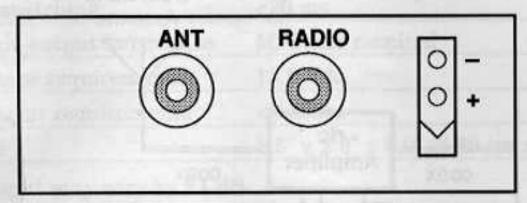
ANT: Antenna. This BNC connector is for connection to a 50 ohm antenna.
