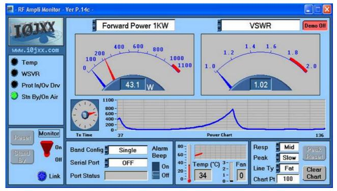
With the switch "Resp" you can change the speed of the response of the analog gauges going to select the preferred between Fast and Slow Mid.
