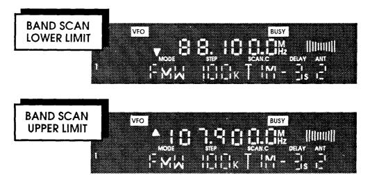
Note: The programming for the commercial FM broadcast band is now complete when MEMO band "1" is recalled. Proceed with the following steps to recall this MEMO band and scan the frequencies.
