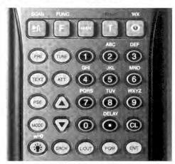
SCAN/▶\ – scans through the programmed channel, or activates the Spectrum Sweeper function.
