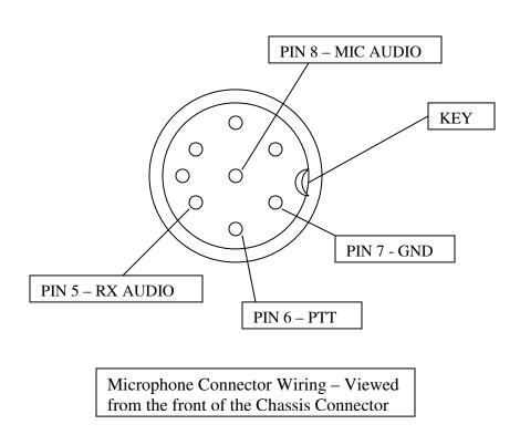
Pin 5 of the connector (RX Audio) is a fixed level audio output from the receiver (not affected by the volume control setting) that can be used for interfacing to a computer to operate digital modes. It is AC coupled to the connector pin but a transformer or optical isolator should be used to couple both the receiver and transmitter audio from the radio to the PC sound card to minimize ground loops and hum on the signals.
