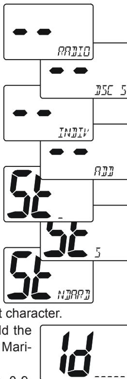
[CALL(SET)MENU] key. Repeat this procedure until all nine space of the MMSI number are entered. If a mistake was made entering the MMSI number, repeat pressing the [SCAN(MEM)] key until the wrong number is selected, then enter the correct number.
