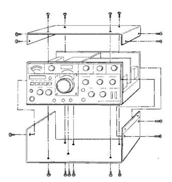
Fig. 23 Removing the Cabinet
