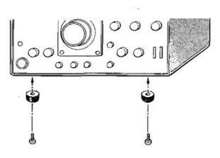
Fig. 31. Attaching the Extension Feet
