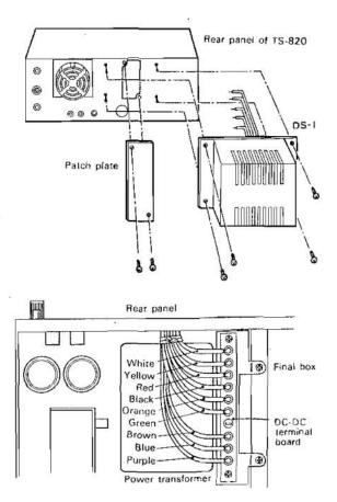
Fig. 26 Installing the DC-DC Converter
