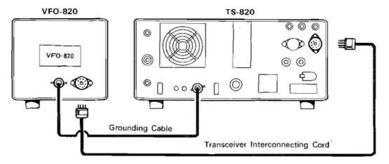
Fig. 29 Connection of Accessory Remote VFO
