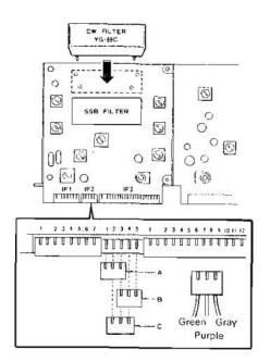
Fig. 25 Installing the CW Filter
