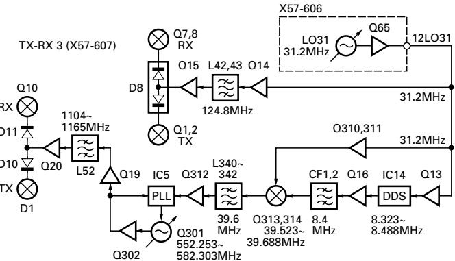
**Fig. 2 1.2GHz unit local oscillator**
