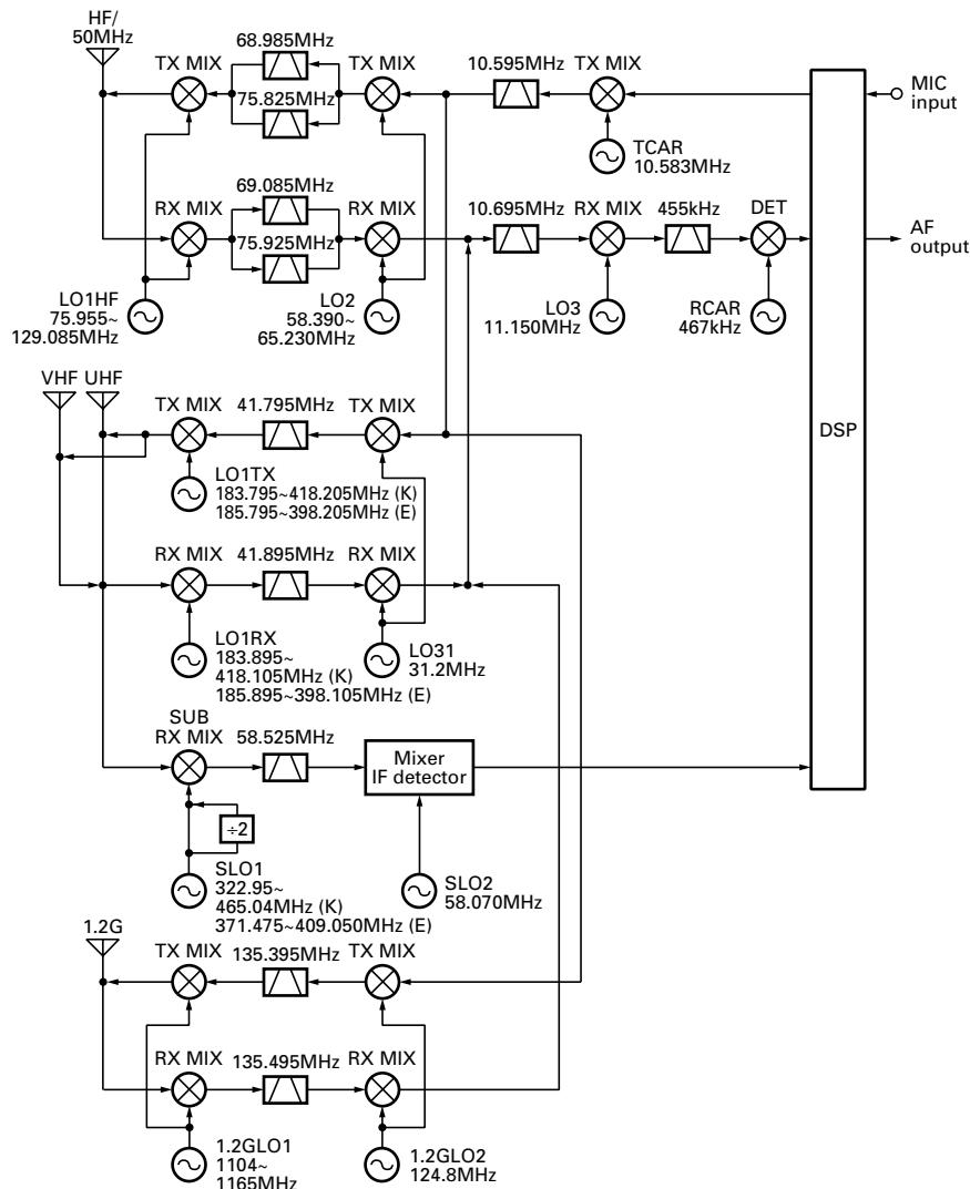
Fig. 1 Frequency configuration
