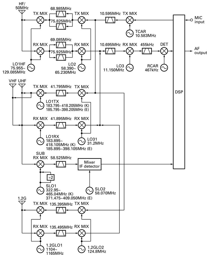
**Fig. 1 Frequency configuration**
