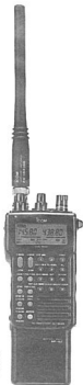
The photo shows IC-W2E with BP-02 BATTERY PACK. The battery pack and antenna differ according to versions.
