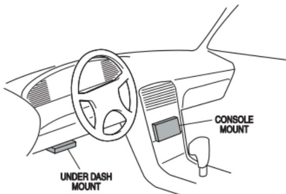
**CAUTION:** Extreme care should be exercised when drilling into the dash to avoid damage to under dash electronic ignition, cruise control, instrument and/or accessory wiring.
