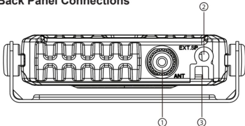
1. **ANT Jack** - SO-239 UHF connector for external antenna (included)
