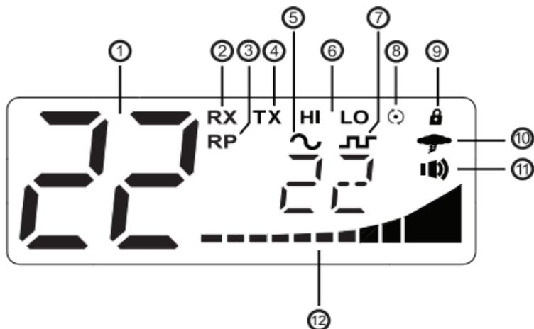
1. **Channel Icon** - Shows the selected transmit/receive channel.
