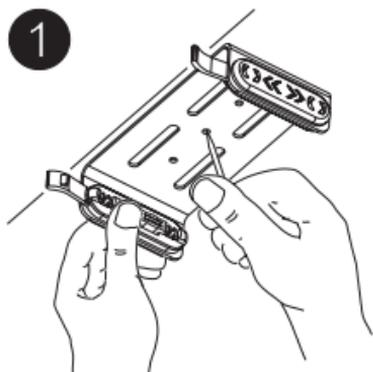
2. Attach the bracket to the dash with the Phillips head sheet metal screws provided. Tighten the screws securely. **DO NOT OVER-TIGHTEN.**
