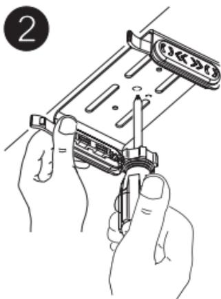
3. Slide the radio into the mounting bracket. **BE SURE** the mounting bracket retainers engage the slots in the sides of the radio to prevent movement while driving.
