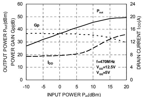
TYPICAL PERFORMANCE ( $T_{case}=+25^{\circ}C$ ,  $Z_G=Z_L=50\Omega$ , unless otherwise specified)
