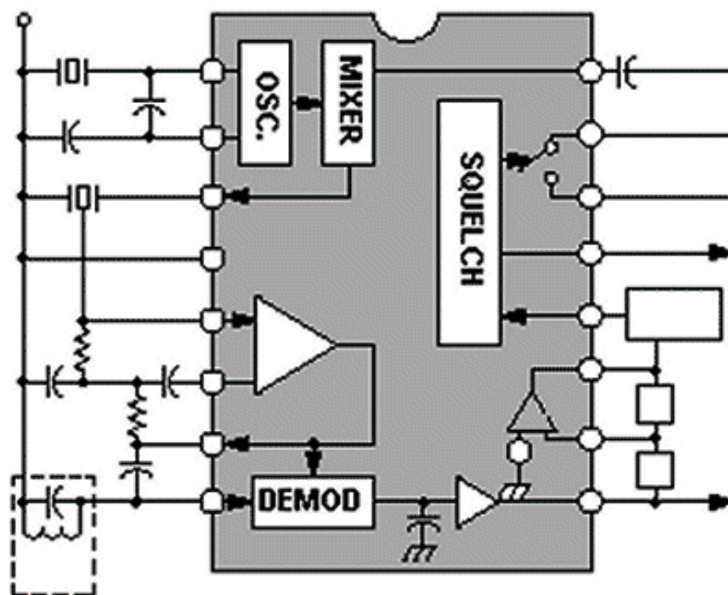
The IR3N06 is a low power narrow band FM detector integrated circuit for FM dual conversion of communication equipment. The IR3N06 includes oscillator, limiting amplifier, AFC circuit, quadrature detect, operational amplifier, squelch circuit, scan-control and muting switch.
