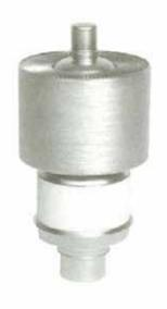
The 3CX3000A7 high-mu forced-air cooled power triode provides relatively high power output as an amplifier, oscillator or modulator at low plate voltages. The tube has a low inductance cylindrical filament tank circuit for VHF operation. Operation with zero grid bias in many applications offers circuit simplicity by eliminating the bias supply. Grounded-grid operation is attractive since a power gain of over twenty times can be obtained.
