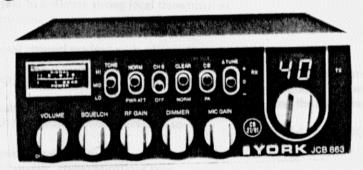
Your York JCB-863 Citizens' Band transceiver is a quality piece of electronic equipment, skillfully constructed from the finest semiconductors and electronic components. The transceiver is loaded with the state-of-the-art circuitry to give you a highly selective and sensitive receiver combined with an efficient 4-watt FM transmitter.
