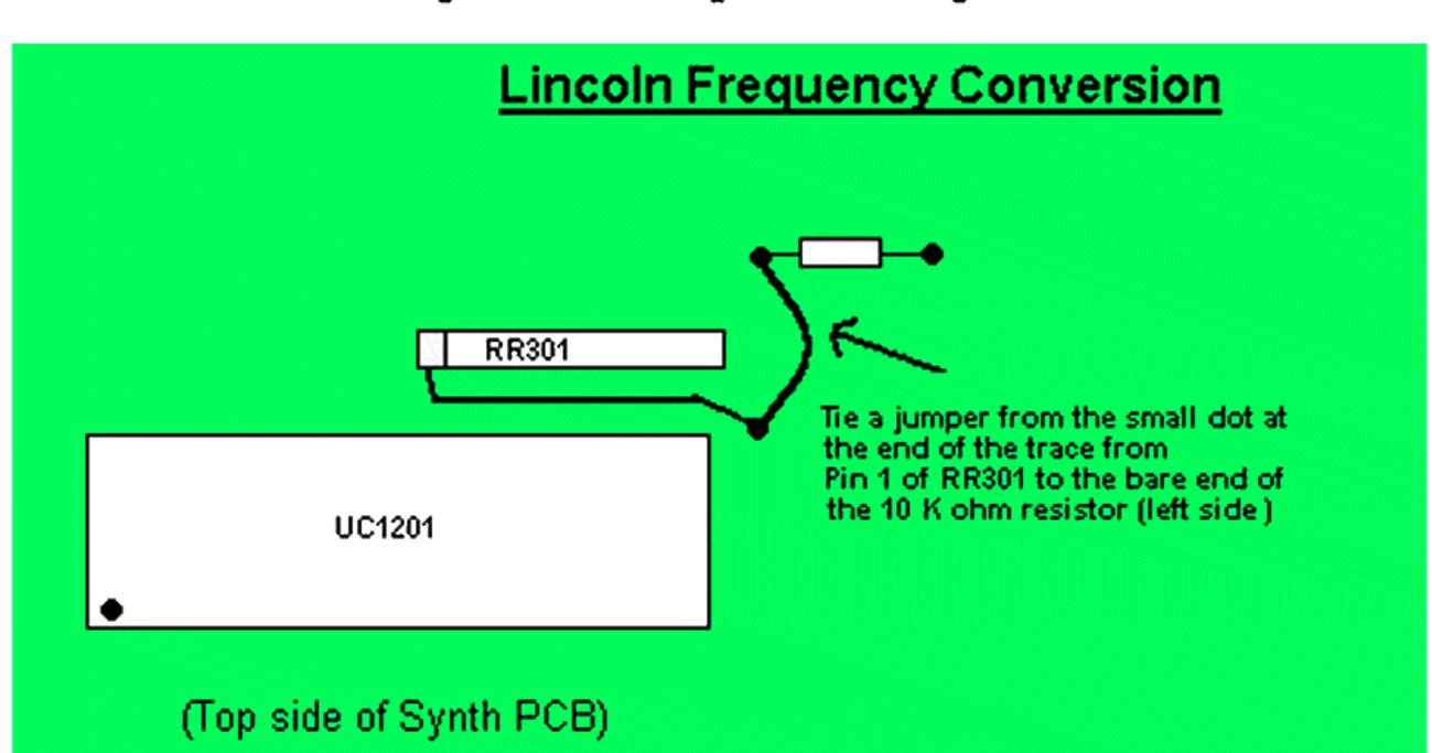
Another mod suggests soldeing a jumper between pins 34 and 35, this will do the same thing. This mod will open the frequency coverage from 26,000 MHz to 29,999 MHz.
