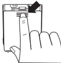
2. Connect the battery pack connector observing the correct polarity.
