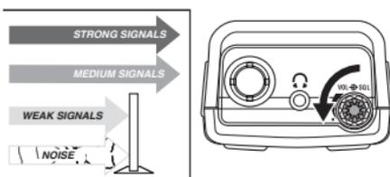
5. Turn **SQUELCH** back counter-clockwise just until the hiss stops. Now the “Squelch Gate” allows only clear signals through.
