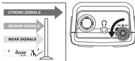
3. Think of the Squelch Control as a gate. Turn the **SQUELCH** control fully counterclockwise. This raises the "Squelch Gate" so high that only very strong signals can get through.
