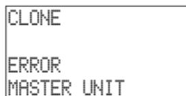
To clear the error, press **○**. To exit the clone mode, repeatedly press **MENU/BACK**.
