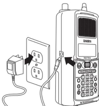
**Note:** Disconnect the AC Adapter/Charger from the unit when charging is complete.
