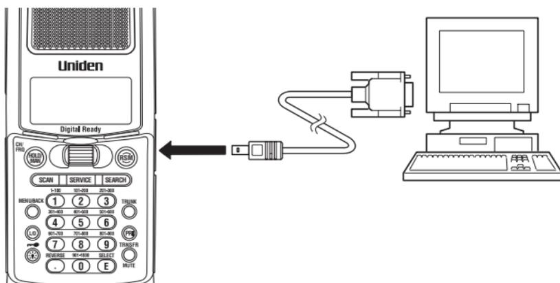
To connect the Scanner to a PC, plug the scanner end of the supplied RS232C cable into the remote port which is on the side of the scanner. Plug the other end of the cable into your PC's serial port.
