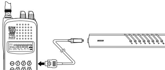
Plug the smaller end of the supplied RS232C cable into the remote port which is on the right side of the scanner. Plug the other end of the cable (DB-9 serial connector) into the external modem. You may need a DB-9 to DB-25 null modem adapter, available at most computer stores. Of course, make sure your external modem is turned on. Make sure that you have a phone line plugged into the modem jack on the back.
