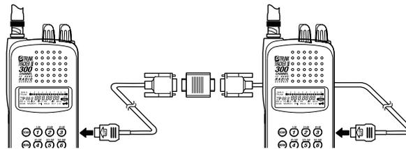
Plug the smaller end of each of the supplied RS232C cables into the remote ports which are on the right sides of each of the two scanners.
