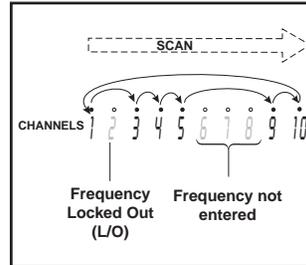
4. When a transmission is received, the LCD back light comes on for five seconds and the scanner stops on that channel, provided that you have selected the Auto Light feature. When the transmission ends, scanning resumes automatically.
