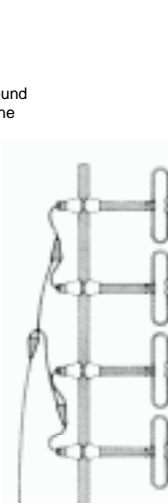
Broad band exposed dipole vertical 6-9 dBd omni used at inband repeaters with duplexer
