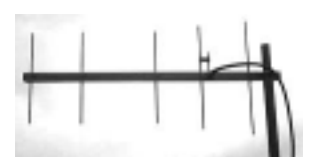
OAL 5L-70cm 8 dBd 420-450 MHz Yagi Mounts horizontal or vertical. 31" boom ideal for portable & public service use
