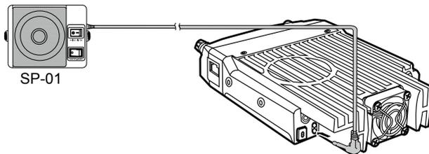
NOTE » External speaker adopt double port BTL, please care about the connecting way. The speaker can not connect with the ground, otherwise the speaker will be damaged. The wrong connecting method as shown in the following diagram.
