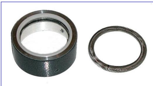
Remove the spring from the collar, if the spring has become deformed, it must be replaced. You can clean the groove that holds the spring with sandpaper. Do not use steel wool. Fibers from the steel wool can contaminate the main coil. One shorted turn on the main coil can cause it to no longer function! Replacement springs are always available here at **High Sierra**.
