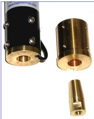
4. Using a wire brush or sandpaper, clean the brass cone shaped surface inside the brass insert in the bottom of the antenna and the brass tapered stud on the mounting bracket. (The base or home version of the mounting bracket does not have a matching coil.)
