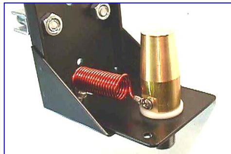
5. Once each year, you should replace the contact spring. That stainless steel spring is subjected to vibration. While many have had the spring last for three or four years, it is prudent to just replace the spring each year. To replace the spring, remove the whip, quick disconnect and weathershield from the antenna. Loosen the three set screws in the collar. Remove the collar.
