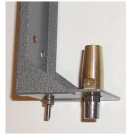
The matching coil is not needed. With radials attached to the screw on the mounting bracket, the antenna will tune to resonance with an impedance close to 50 ohms.
