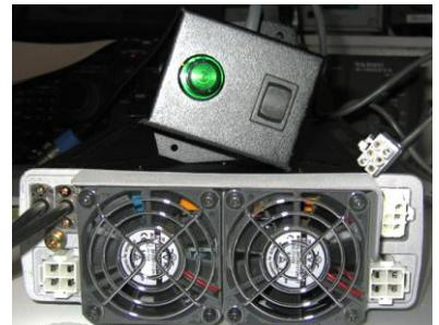
We have provided the plug for the wires to the motor. You can simply use butt connectors to make the connection to the wires that go to the antenna’s motor.
