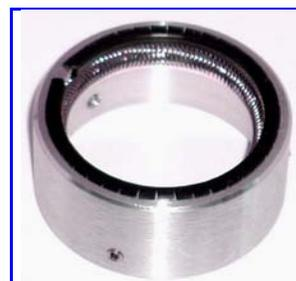
Over time (and especially in salt water environments) you may find some aluminum oxide build-up under the spring in the 'decoupler.' Simply remove the spring and clean the aluminum surface with steel wool. Put a *small* amount of an antioxidant (such as NO-OX) in the groove before replacing the contact spring. A 'Q-Tip' cotton applicator works well for this purpose.
