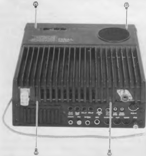
Figure 5: Local Unit Shield Cover
