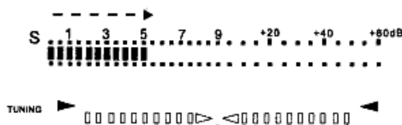
Tune for Maximum Signal Strength and Centered Marker Segment
