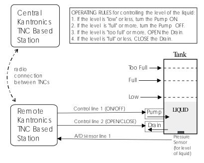
Example: controlling the level of liquid in a tank
