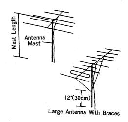
NOTE: Cut antenna mast 12"(30cm) longer than distance needed to mount antenna and brace.
