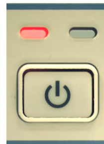
EB500 without front control panel in Failure mode. Refer to the Troubleshooting section in the Operating Manual for possible actions to take.
