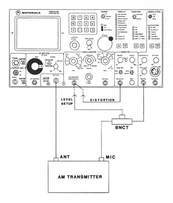
FIGURE 4-12. AM MODULATION TEST SETUP
