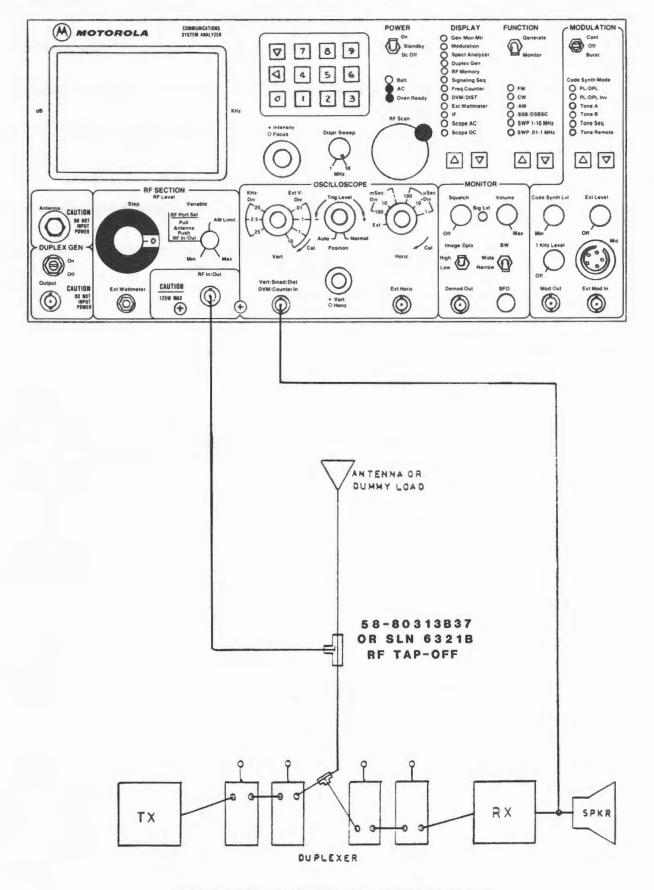
FIGURE 4-24. DESENSITIZATION TEST SETUP
