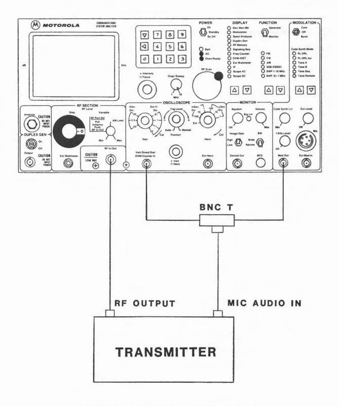
FIGURE 4-10. AUDIO FREQUENCY RESPONSE SETUP
