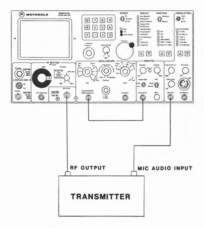
FIGURE 4-9. AUDIO DISTORTION SETUP
