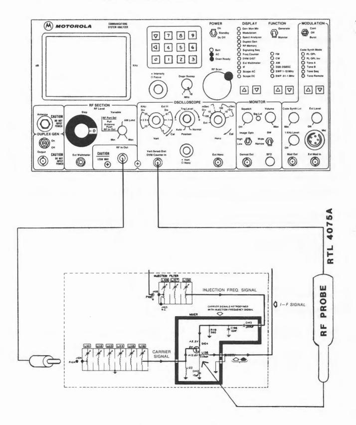
**FIGURE 4-5. PROBE SETUP**
