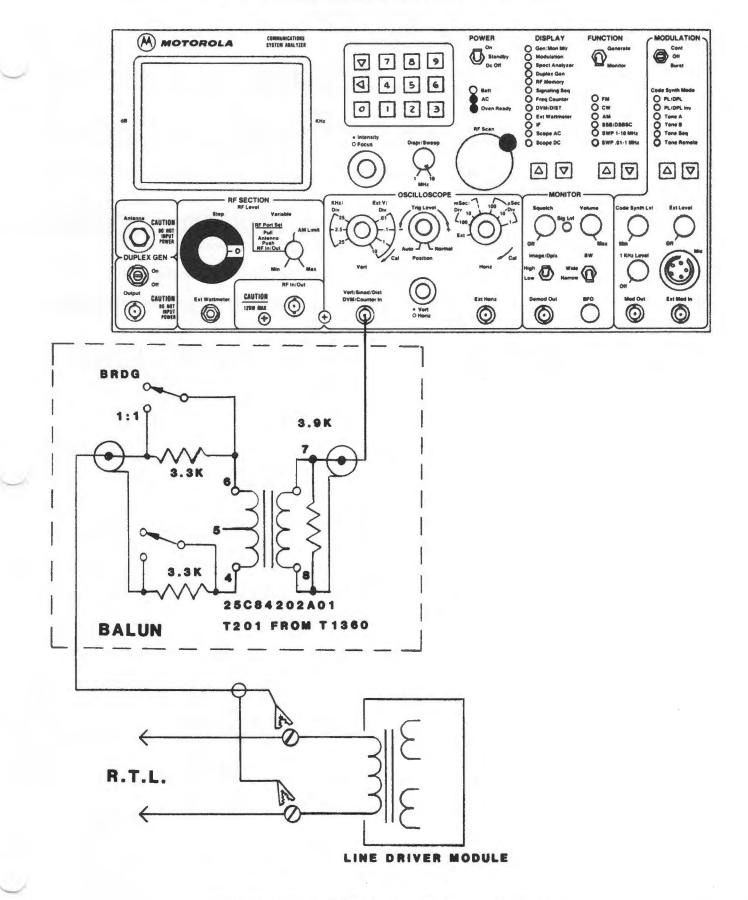
FIGURE 4-18. BALUN SETUP; MEASURING LEVELS
