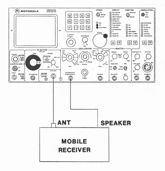
FIGURE 4-3. SQUELCH SENSITIVITY TEST SETUP
