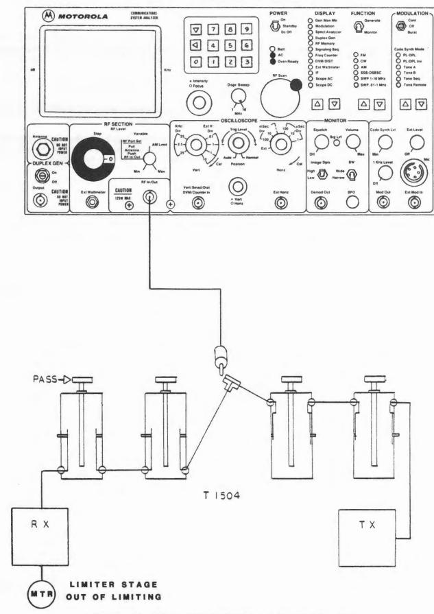
FIGURE 4-21. DUPLEXER PASSBAND ADJUSTMENT SETUP
