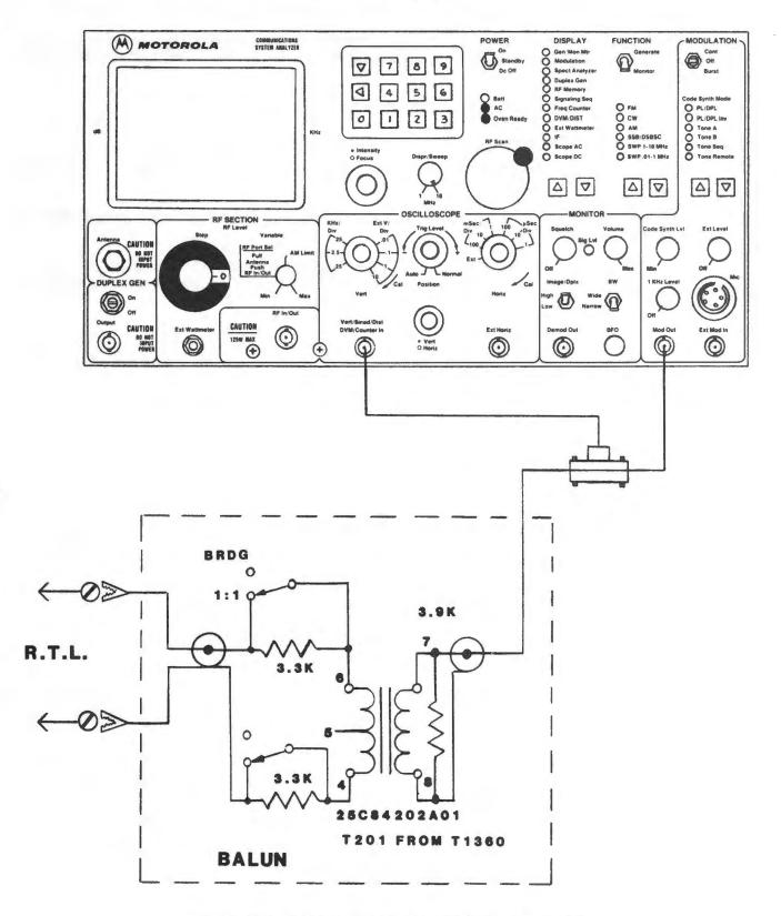
FIGURE 4-19. BALUN SETUP; GENERATING SIGNALS
