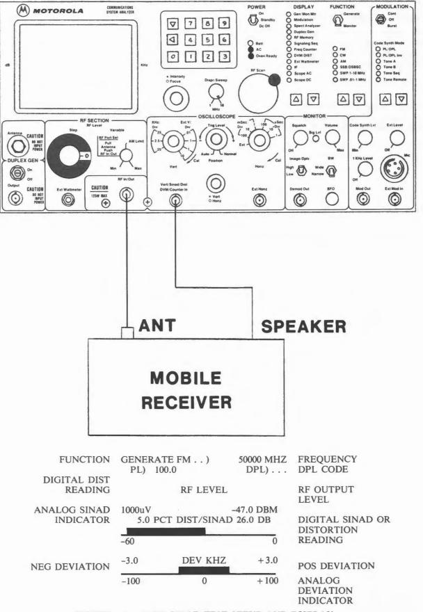
FIGURE 4-1. 12 DB SINAD TEST SETUP AND DISPLAY
