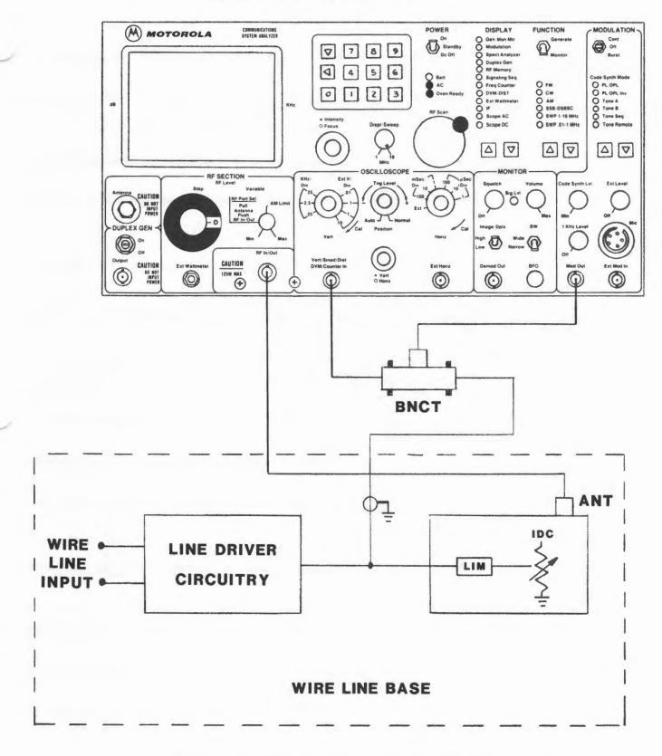
FIGURE 4-16. MODULATION SETUP; REMOTE BASE
