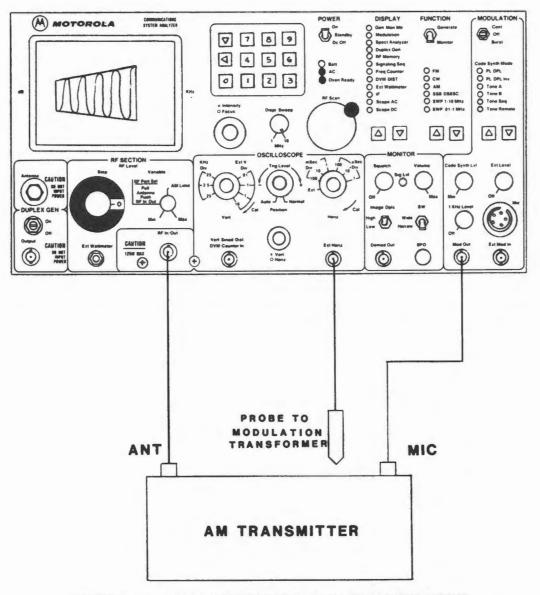
FIGURE 4-13. AM MODULATION LINEARITY TEST SETUP
