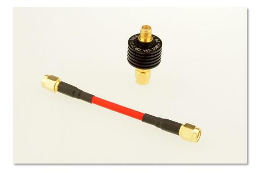
HINT: Since SMA connectors are easily damaged by repeated connection/disconnection, it is recommended to connect the attenuator directly to the power meter, and use the SMA adapter to connect to the RF source. The adapter will be much cheaper to replace than the attenuator, if the connector is damaged.
