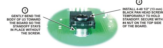
Figure 2. Installing U3 Spacer.
