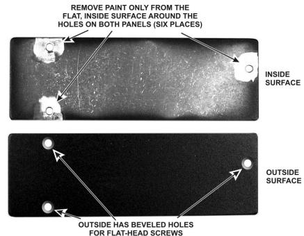
Figure 11. Preparing the Side Panels for Mounting.
