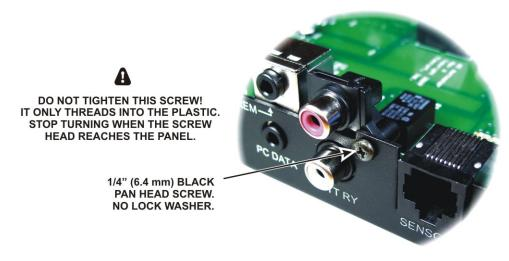
Figure 8. Installing PTT RY Connector Screw.
