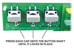
Figure 4. Installing Pushbutton Key Caps.
