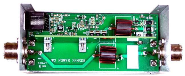
Figure 13. Typical Directional Coupler Sensor Interior View.
