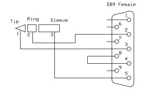
Above is the schematic diagram of the optional RS232 serial interface cable. A kit of parts to assemble the cable is available from Elecraft (order W1SERKT), or you can order a factory-assembled cable from Elecraft (order KXSER). If you order the KXSER cable, it may arrive in a bag marked E850369.
