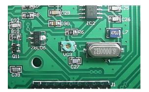
Adjust signal generator frequency to 14.100Mhz or close to frequency, put EK-1B on same frequency, now adjust VC2 to max the receiver sensitivity.
