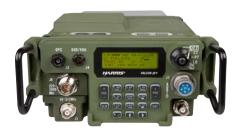
Software defined, with a JTEL-certified Software Communications Architecture (SCA), the fully JTRS-compliant Multiband Networking Manpack supports in-field upgrades as new capabilities emerge. The AN/PRC-117G is MUOS-ready, extending critical communications Beyond-Line-Of-Sight (BLOS) with simultaneous SATCOM voice and data.
