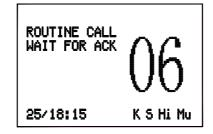
When a reply is received, the radio will sound a tone and automatically switch to the specified working channel. A voice call can then be made in the normal way.
