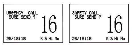
Press the **(ENT)** key again to make the call, or press **(CLR)** to cancel. When the call is sent, the radio will be set to the working channel. Allow a few seconds for the stations receiving the call to switch to the working channel. Then make a normal voice call on the selected working channel.
