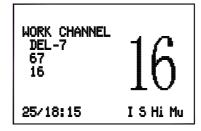
Press  $\blacktriangleleft$  or  $\blacktriangleright$  key to select the channel (5th – 9th channel) that you wish to delete, then press **(ENT)** key to accept.
