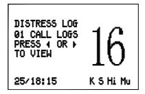
If there are any distress calls in the distress log screen, press the ◀ or ► key to move back and forth through the DISTRESS LOG screen. The DISTRESS LOG screen as below:
