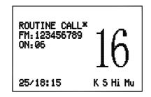
Press the **(ENT)** key on the fist/mike keypad, an acknowledgement will be sent to the caller and the radio will be automatically switched to working channel for normal voice communication. The "\*" will disappear when the call has been acknowledged.
