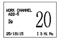
Press  $\blacktriangle$  or  $\triangledown$  key to change the selected channel, and press (ENT) key to accept. Then press  $\blacktriangleleft$  or  $\triangleright$  key to enter the next channel.
