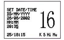
Use the numeric keys to enter numbers, then press **(ENT)** key to confirm the date and time.
