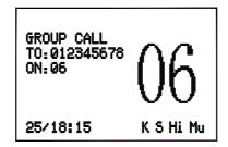
Select a working channel from the channel list by pressing the  $\blacktriangle$  or  $\blacktriangledown$  key on the keypad.
