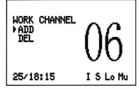
Press  $\blacktriangle$  or  $\lor$  key to select "ADD" from the WORK CHANNEL screen, then press **(ENT)** key to enter, as below:
