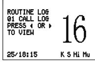
If there are any general calls in the routine log press the ◀ or ► key to move back and forth through the log, the ROUTINE LOG screen as below:
