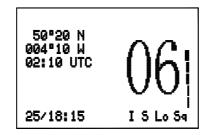
Then use  $\blacktriangle$  and  $\blacktriangledown$  key on the front panel to adjust the receiver muting threshold (squelch) level.
