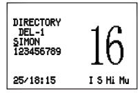
Use the  $\blacktriangleleft$  or  $\blacktriangleright$  key to move along the name and MMSI fields, using the soft keypad to edit the data. Press **(ENT)** to store the modified entry.
