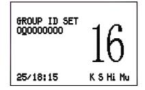
Press numeric soft key to enter the GROUP ID number (8-digits, the first digit must be "0"). If a mistake is made, use the  $\triangleleft$  or  $\blacktriangleright$  key to move back the cursor and reset the number. Press **(ENT)** key and the radio will ask for verification. Check that the no, is correct and press **(ENT)** key once again to confirm your entry. To amend, press **(CLR)** key to go back to main screen.
