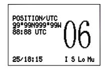
Use the numeric soft key to enter the required data, then press **(ENT)** key to accept the position and time entered.
