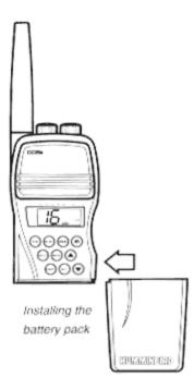
When the battery pack is off the DC5s unit, care should be used to prevent damage to the mating slide and electrical contacts on the top of the battery. Also the slide and contact area on the bottom of the unit will be vulnerable to damage if not protected. It is best to keep the battery pack installed even if the radio is being stored for extended periods.
