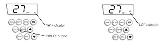
Selection of certain channels will cause the DC5s to automatically select the LO power output. This feature is required by the FCC.
