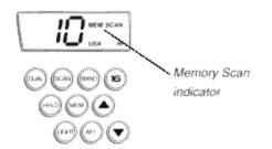
To delete a channel from Memory, select the Memory function and ensure the MEM enunciator is displayed. Use the Up or Down arrow button to select the channel to be deleted, and press M+/-. The channel is now deleted from memory.
