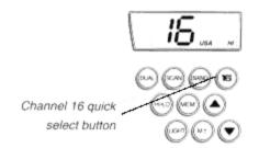
Channel 16 represents the same frequency on both USA and INT bands. If 16 is pressed again, the DC5s will return to the previously selected channel.
