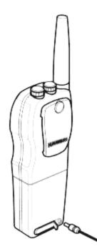
The battery drain is considerably greater when transmitting than receiving. A battery charge can be maintained for 8 hours or more (depending on ambient temperatures) when receiving only. Frequent transmitting, especially on High (5 Watt) output power will significantly increase the battery drain.
