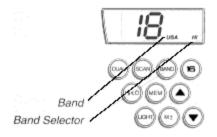
Pressing the BAND button will toggle between these three bands. As with all controls, an audible chirp will be heard when the button is pressed.
