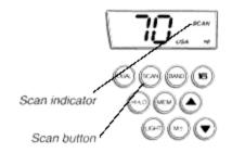
Pressing the SCAN button again will disengage scan.
