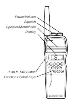
Most control inputs result in audible, tactile, and visual feedback for positive actuation in loud environments.
