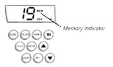
By pressing MEM, the Memory function is selected and the MEM enunciator will be continuously displayed. When in the MEM function, only channels stored to Memory will be accessible. The Up and Down arrow keys can be used to select any channel stored to memory. SCAN can be used to scan only the Memory channels.
