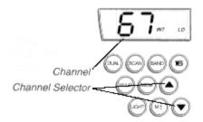
Within each of these three bands there are a number of discrete channels. These channels are selected using the UP and DOWN arrow keys. Pressing either key once will select the next higher or lower channel. Pressing and holding either arrow key will scroll through all available channels.
