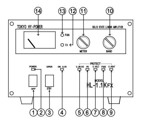
**POWER** : Main power switch to turn AC power on and off.
