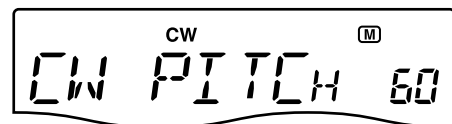
This shows the default setting for the CW tone pitch control (600 Hz).
