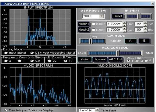
Display of the tuned AM signal together with a CW interfering signal. (Interfering signal 1Khz down of the carrier frequency)
