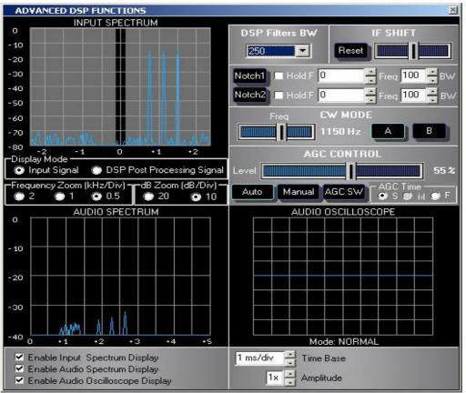
*Mode B CW demodulation with fixed BFO and Zero beat. To hear the 800 Hz Audible tone a different VFO tuning will be required.*
