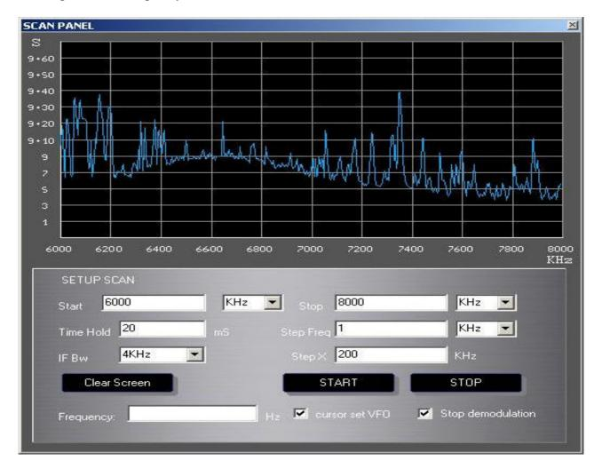
At the end of the scanning process a diagram with S-meter level and frequencies will be displayed. Passing with the mouse over the diagram the relevant frequencies will be displayed on the frequency windows located on the left bottom side. Left clicking with the mouse on a point in the diagram a red mark can be inserted and the relevant frequency will be tuned and displayed on the cockpit.
