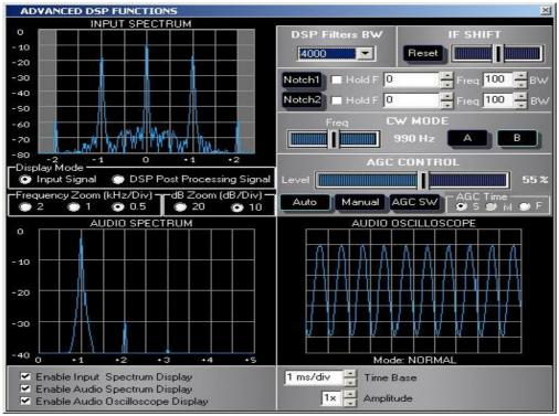
AM signal received with 4.0 KHz BW DSP filter
