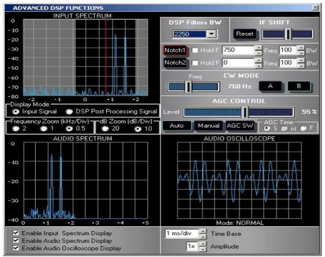
Thanks to filter notch 1 the interfering signal at 750 Hz has been eliminated.
