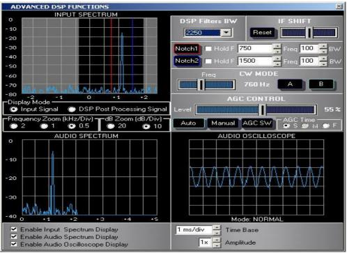
Both interfering signals have been eliminated using notch 1 and 2
