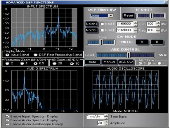
USB signal received with 2.5 KHz BW DSP filter
