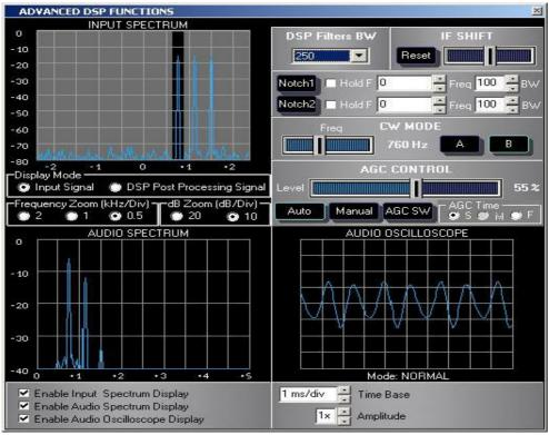
Mode A CW demodulation using BFO for 800 Hz audible tone.
