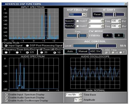
Mode A CW demodulation using BFO for 1.100 Hz audible tone.
