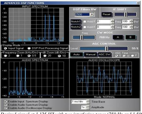
Desired signal at 1.125 HZ with two interfering tones (750 Hz and 1.500 Hz).
