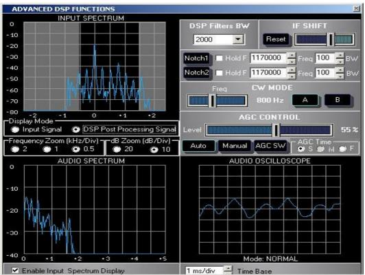
IF band pass filter shifted 500 Hz up to attenuate the CW interfering signal.
