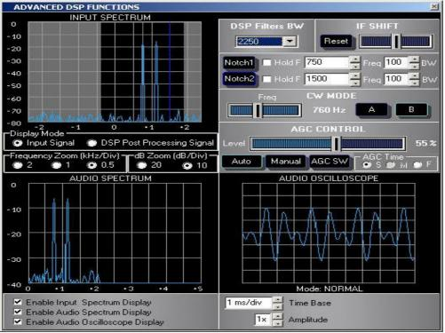
Thanks to filter notch 2 the interfering signal at 1.500 Hz has been eliminated.
