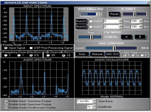
FM signal received with 5.0 KHz BW DSP filter.
