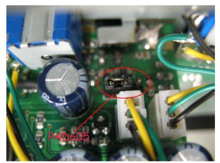
With this modify the radio will work on 400 channels in 10 bands, from 25.615 MHz to 30.105 MHz; the display will show from A 01 (lower frequency) to L 40 (higher frequency).
