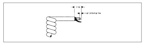
**Fig. 2.** Microphone Cable Preparation. To wire the microphone cable to the plug provided, proceed as follows:
