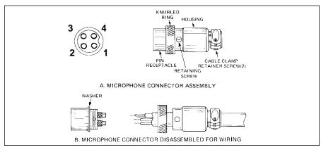
Fig. 3. Microphone plug wiring.
