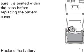
7. Replace the battery cover by putting the two tabs in the corresponding opening and sliding it upward until it locks in place.
