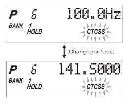
4. Press E to program the tone with the frequency stored in the channel.
