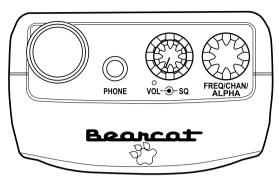
Antenna Connector Connect the rubber antenna to the BNC connector and turn clockwise until it locks.
