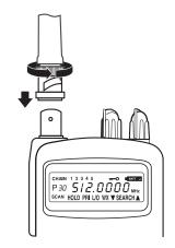
Attach the flexible antenna to the **BNC** connector.
