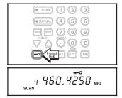
To unlock the keypad, press and hold —o until the key symbol disappears.
